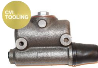
87694 Brake master cylinder, PV/ Duett 1947-1959
