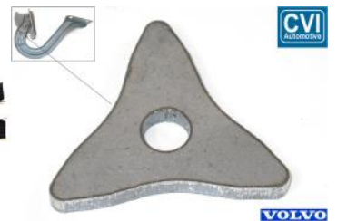
91693-1 Starwheel bootlid hinge, PV LH
